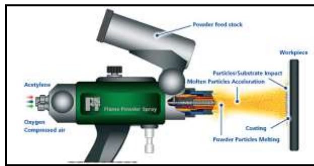
Figure Flame Spray Thermal Spray Coating
